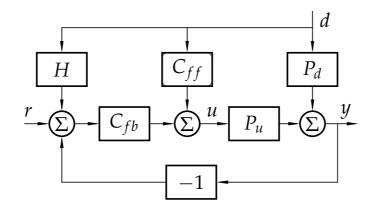
$$e = \frac{r + (H - P_d + P_u C_{ff})d}{1 + P_u C_{fb}}, \ H = P_{ff} = P_d - P_u C_{ff}$$
