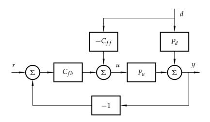
$$y = \frac{P_d - C_{ff} P_u}{1 + L} d = \frac{P_d - C_{ff} P_u}{1 + C_{fb} P_u} d$$
