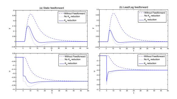
The feedforward gain  $\kappa_{ff}$  has been reduced from 1 to 0.778 for the static feedforward and from 1 to 0.889 for the lead-lag filter.
